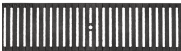
Slotted grating, HEELGUARD , cast iron, coated in black Load classes: D400*, Length: 50 cm, SW 6 mm
