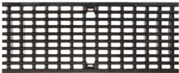
Longitudinal Grating , cast iron GJS Load classes: D400*, E600*, Length: 50 cm, MW 25 x 11 mm
