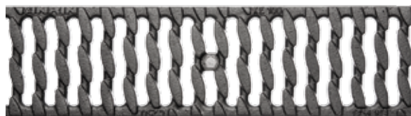
Slotted grating, Oval Grip Design , cast iron, cataphoretic dip coating Load classes: C250, E600*, Length: 50 cm, SW 10 mm
