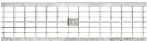
Mesh grating , galvanised, stainless steel Load classes: B125, C250, D400, Length: 50 cm, 100 cm MW 30 x 14 mm / 30 x 10 mm / 20 x 14 mm
