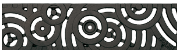
Design grating, CELTIC , cast iron, cataphoretic dip coating Load classes: C250, Length: 50 cm, SW 10 mm
