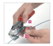
13 Remove multifiber buffer tube piece (sliver) with sharp sidecutter
